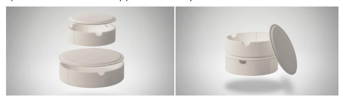
**UltraSaggar UV 1600-10** are saggars, optionally with lid, for sintering and firing small-sized products. They are made of polycrystalline mullite fibres (PCW). The product is perfectly usable up to 1600°C application temperature. Thanks to their material properties, rapid and frequent temperature changes can be perfectly realized. A wall thickness of 4-7 mm (depends on the outer diameter) provides optimum heat transmission.
