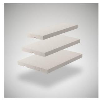
**UltraSetters UV 1700-10** are lightweight sintering and firing setters based on polycrystalline mullite fibres (PCW). They are suitable for application temperatures of up to 1650°C (geometry dependent) and serve as stable setters in many application areas where sintering, firing or heat treatment processes take place.
