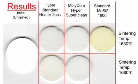
Fig. 5: Color changes from different heating element qualities.
