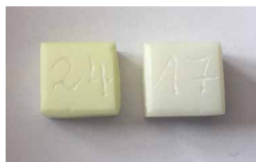
Fig. 9: Sample 24 was sintered on a closed Saggar (muffle). Sample 17 was inside the Saggar in the same firing run in a contaminated furnace.
